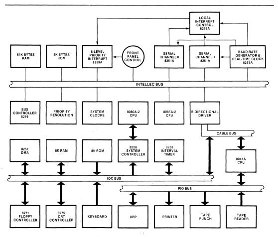
Figure 1. Intellec Series II/85 Model 225 Microcomputer Development System Block Diagram
